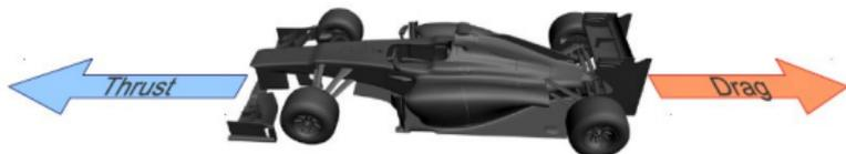
Infer power and drag based on noisy *acceleration measurements* using a simple inertial and aerodynamic model
